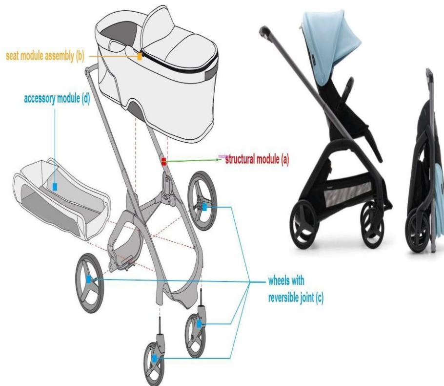
Figure 4. Modular structure of the Bugaboo Dragonfly pushchair
