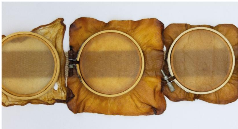
Figure 3. From the left: 4 mm thickness BC film, 7 mm thickness BC film, and 10 mm thickness BC film
