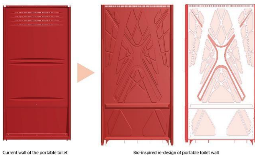
Figure 6. Side walls compared: on the left front view of the current component, on the right the component re-designed bio-inspired. Image owned by the authors
